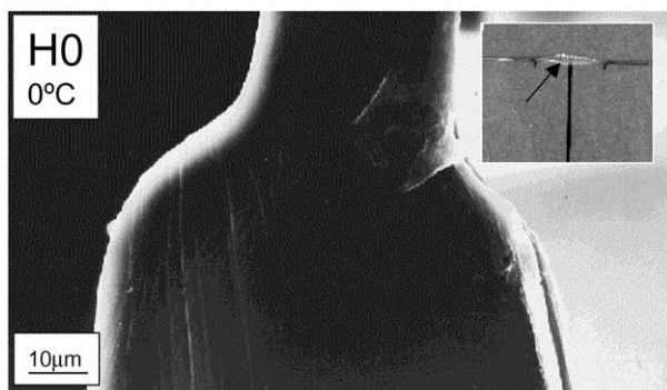
Fig. 10. SEM micrographs of the section of a H0 specimen tested at 0 °C, showing the neck region (the arrow in the inset shows the exact point where the image was taken from).
